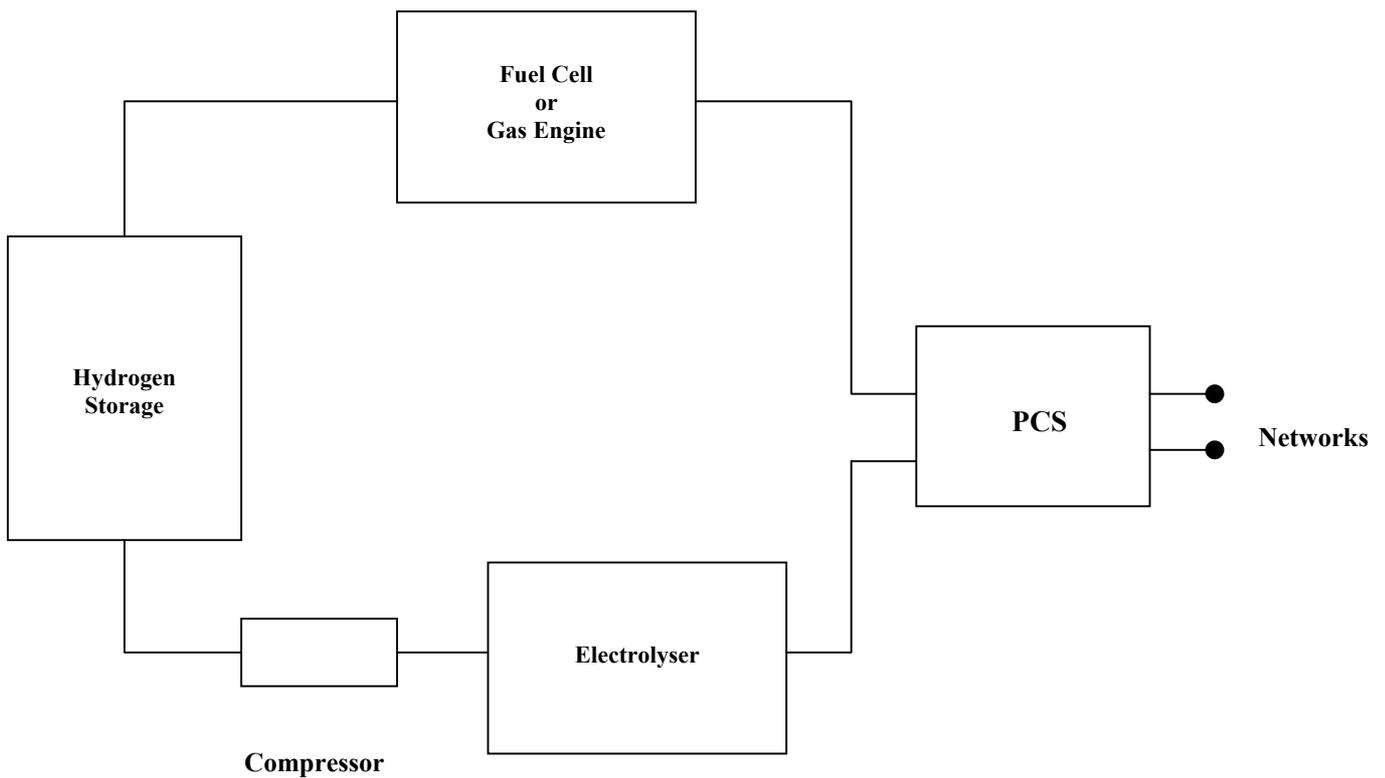
**Figure 6.1 Diagrammatic Representation of Hydrogen Energy Storage System**
