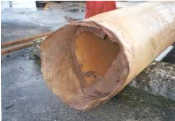
**Fig. 4-5: Point of fracture of FRP string**
